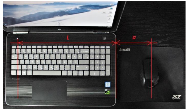
Fig 4. A graphic display of the dimensions required to calculate the average hand transfer distance
